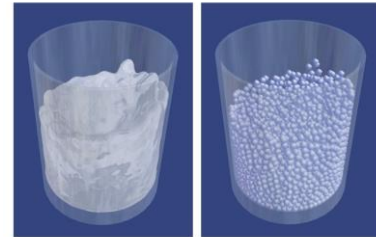
Figure 1 – A volume of fluid is rendered as a continuum (Left) and as discretized particles (Right) (Müller, Charypar and Gross 2003).
