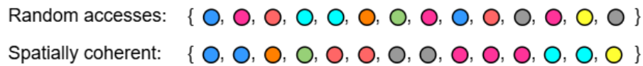
Figure 11 - Order of particle memory access. Random memory reads (Top) and spatially coherent reads (Bottom).
